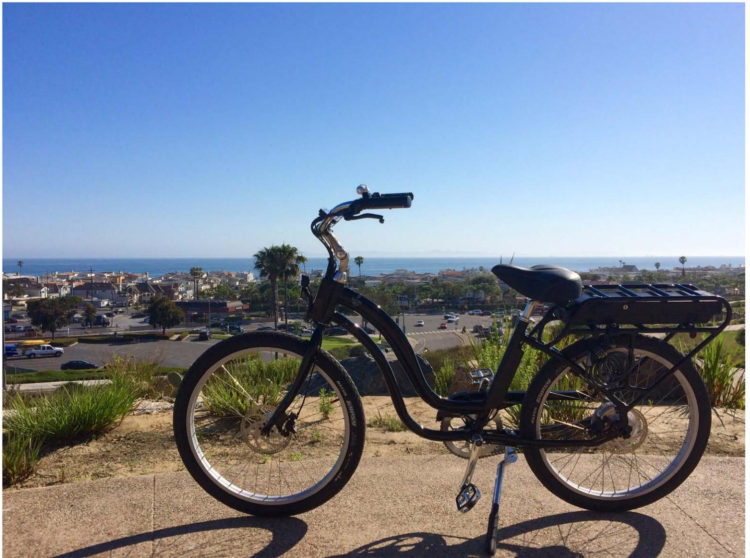
The power available from the bike's "500 watt rated" motor is very impressive. Even at low power settings it felt like it was as much as I would ever need or want. While riding, the bike's computer allows fairly easy switching between 5 levels of strength and turning pedal assist on and off. The battery/controller/motor are technically capable of putting out up to 1300W for short bursts, but only rated for 500W for an extended period of time. Typical riding will use ~200-300W.
